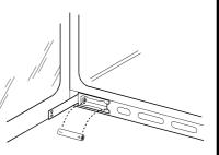
When you fit the new battery, make sure the positive end (marked with a + sign) is next to the (+) sign on the battery holder. Close the lid of the battery holder.
